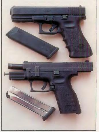
To fieldstrip the XD pistol (bottom) the slide must first be locked to the rear to rotate the disassembly lever, and this automatically ejects a round from the chamber, a great safety feature.
